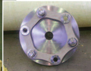
AISI 301 disc-pack with an antifretting and anti-rust coating.
