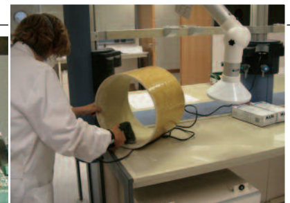
Superficial treatment for composite shaft
