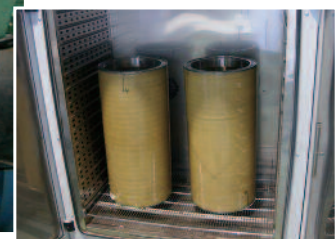
Bonded joint curing
